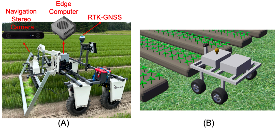
Fig. 1. A stereo vision-guided UGV for bareroot forest nursery inventory. (A) Physical UGV. (B) Webots simulation.
